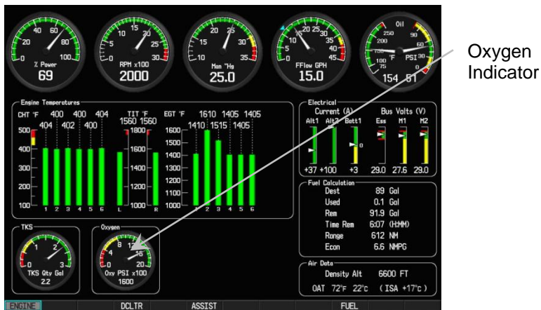
Figure 4 – Typical Cirrus Perspective MFD Engine Page
